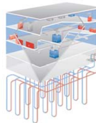
Figure 3. A typical closed-loop, commercial geoechange system.
